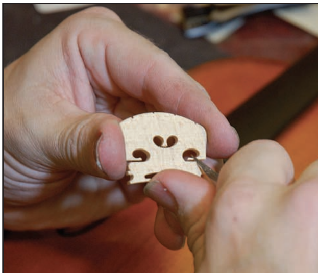
Veteran luthier David Wilson (above), who has been with Hammond Ashley since 1973, repairs a crack in a double bass. Such exacting work often requires the use of unique tools, many of which Wilson builds himself. Every violin that Hammond Ashley sells gets a new custom-made bridge (right), hand carved from high-quality European maple.
